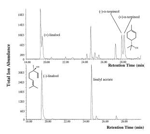
Fig. 4. Chiral chromatograms of Tasmanian lavender oil, showing the simultaneous resolution of  $(\pm)$ -linalool, and  $(\pm)$ - $\alpha$ -terpineol (upper trace). These additional components result from racemisation and rearrangement during acid hydrolysis of the original oil, which is enriched in (-)-linalool (lower trace). The enantiomeric composition of  $\alpha$ -terpineol was 56% (+)- and 44% (-)-.
