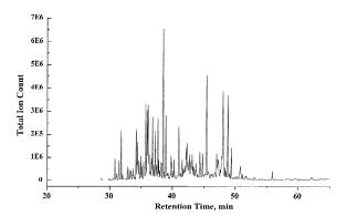
Fig. 10. Typical analysis of *Vetiveria zizanioides* (vetiver) oil by using GC–MS analysis. Agilent 6890GC with a 5730 mass-selective detector, and a BPX5 capillary column (SGE International). Temperature program of 45°C, held for 6 min, then temperature programmed at 3°C/min to 250°C. Initial column head pressure 3.47 p.s.i. (constant flow mode; 1 p.s.i.=6894.76 Pa).
