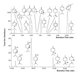
Fig. 3. The monoterpene hydrocarbon and oxygenated monoterpene region (upper and lower traces, respectively) of a chromatogram (determined on a commercial chiral column, J&W CyclodexB,  $30~\text{m}\times0.25~\text{mm}$  I.D.,  $0.25~\text{\mu}\text{m}$  film thickness) from a typical sample of flush growth from *Melaleuca alternifolia*.
