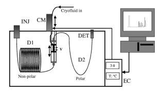
Fig. 9. Schematic diagram of the GC $\times$ GC arrangement utilising a cryogenic modulator. CM: Cryomodulator; INJ: injector; DET: detector; D1, D2: separation dimensions 1 and 2; EC: electronic controller with selectable modulation duration (30=3.0 s) and cryotrap temperature shown; V: exit vents from the cryotrap. The modulator oscillates as shown by the arrow. Cryofluid CO $_2$  is provided to the trap via the movement arm.
