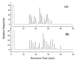
Fig. 2. Illustration of expanded separation space when using a more "selective" column. (A) Compounds are restricted to a small elution (temperature) range for example with a non-polar column. (B) By using a polar (selective) column, compounds with polar groups are retained more strongly and so the total sample will be spread over a greater elution range. This leads to better apparent resolution.
